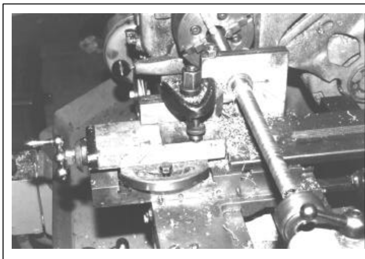
Top-slide turned through 90 degrees to index tool
